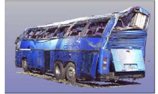
support structures. Using 3D laser scanning technology, National Transportation Safety Board (NTSB) investigators documented the accident scene and the motorcoach. (See image).
